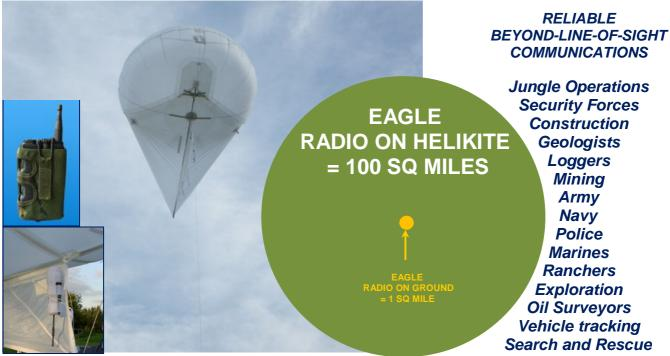
Mobile Ad-Hoc Network (MANET) radios such as the latest Cobham Eagle PRR Radio, carry substantial encrypted information including voice, data, GPS. However the high band width, high frequency, low-power, radio waves required for this cannot bend around terrain. Without a high altitude relay they are generally restricted in range to a few hundred yards, typically less than one square mile.
