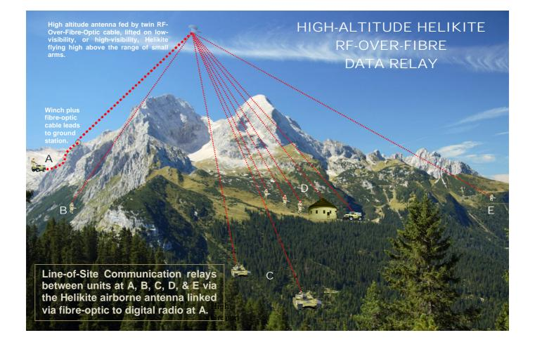
Airborne component of PPM RF-Over-Fibre radio-relay system.
